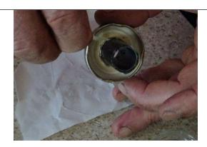
Use your mixing tool to place analdite around the joint inside and out to fix the tub in place and for a seal round the tube.
