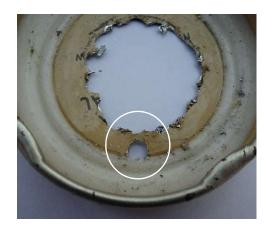
5. Drill one more hole just outside the main hole with a 2 or 3mm drill. This acts a pressure relief hole when hot sunshine heats air and liquid inside the jar. If there is no hole then liquid is pushed up the tube by the increase in pressure and this spills out all over the lid.
