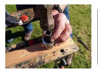
7. Screw the lid on to the jar and using a hammer and so long as the hole is close in size to the tube you should be able to tap the tube down through the hole. The ragged edges of the hole will grip the side of the tube so you can adjust how far down the tube goes. Try to get the tube siting about 5mm from the bottom of the jar.
