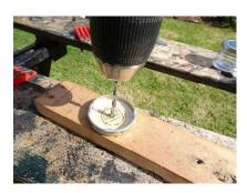
3. With a spare piece of softwood under the work (don't drill directly on you table or work top), drill a small hole (4mm or so) and use this hole for a screw to fix the lid to the wood.
