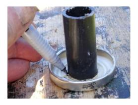
2. On the inside of the lid use the tube to mark out where the hole is to be made. I have used an overhead projector pen as the ink "sticks" to the metal and gives fine line.
