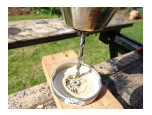
4. "Chain Drill" round the <u>inside</u> of the circle with a small drill. Sometimes the drill will overlap the previous hole. You can also tilt the drill into the previous hole once you have gone through the metal, thus linking the hole into a continuous slot.
