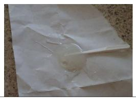
8. Five minute setting Araldite (or a similar epoxy resin adhesive) is best for the next step so mix up equal parts of adhesive and hardener on a piece of card or thick paper. I use plastic dental picks as mixing and spreading tools.
