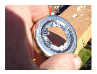
6. You will find you have to tap the drilled edge of the hole flat with a hammer from the inside of the lid on your spare piece of softwood.
